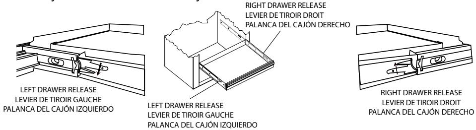
To maintain the smooth and quiet operation of the ball-bearing slides, lubricate the extension track that houses the ball bearings every 3-6 months with a high quality jelly-like petroleum based lubricant.
