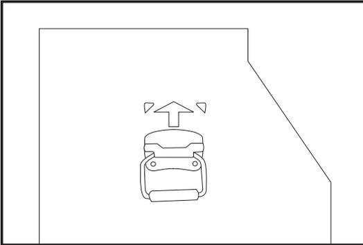
Slide lift handle (Part A) into slits and use 2 screws from Hardware Bag (part E) to secure to Canopy. There is one handle on each side.
