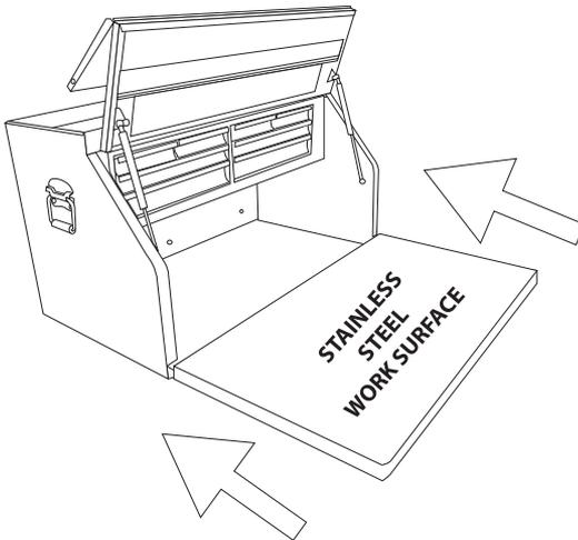
To install Stainless Steel Worksurface (\*Included with 42" Black Satin Roller Cabinet) Use Two People to Slide the board into the slits at the bottom of the canopy.
